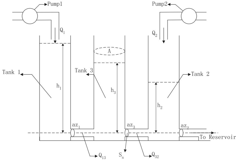
Figure 2. Three-tank system DTS200 (Xie et al., 1999).
