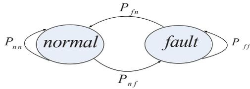
Figure 1. Intermittent faults described by Markov chain.
